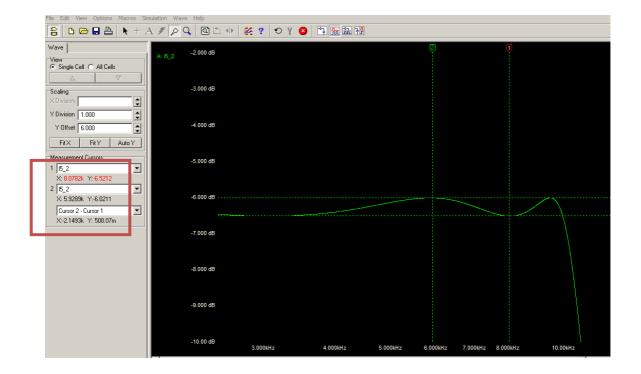
The corner frequency of our filter is shown in the plot below.
