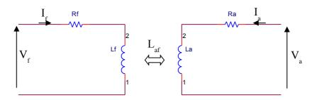
To compute the speed of a DC machine from the load it carries during its steady state operation, a total of two equations will be used. The first gives the relationship between the magnitude of the back EMF at the armature, the speed of the machine, and the field current.
