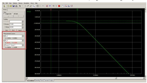
We see that the 3dB point of our circuit occurs around the 3.2kHz frequency.
