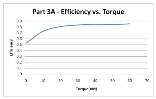
From the plot, it can be seen that efficiency increases as the load torque increases up to a certain limit. At which point, the efficiency of the DC machine reaches a plateau.
